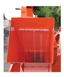
Extra large 10" x 14" infeed opening means less pruning and trimming! Debris curtains help protect operator from fly back of material.
